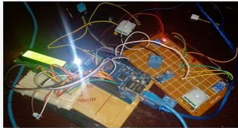
Figure 13 Prototype of the Power Optimization System with Fuzzy Inference System
