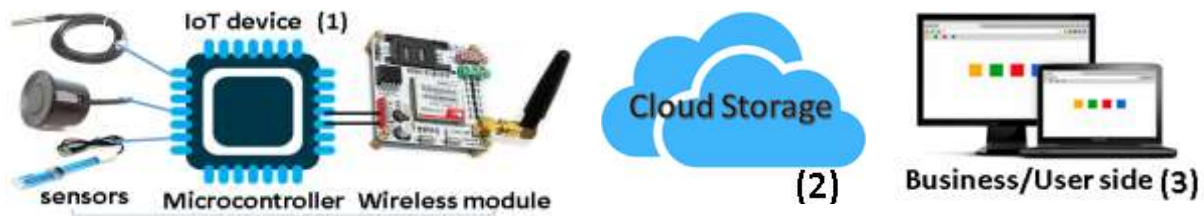
Figure 12: Three main sections of system
