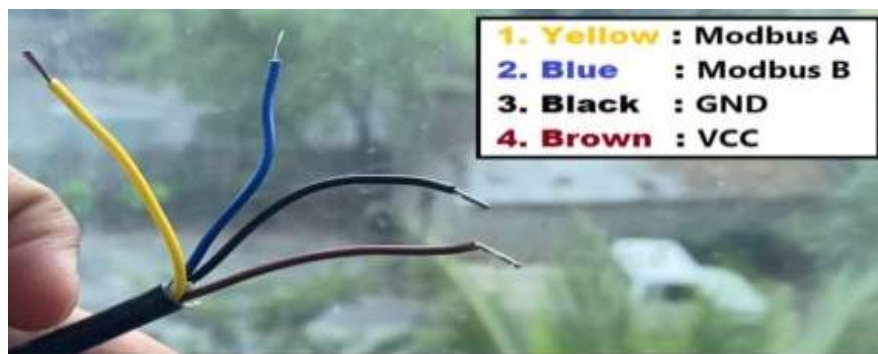
Figure 4.6: Pin connection of soil pH sensor to the interface module
