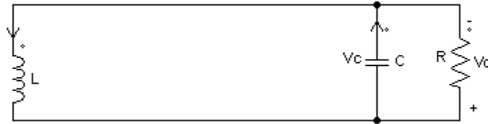
Figure 13: Equivalent of Buck-boost converter if the switch is off
