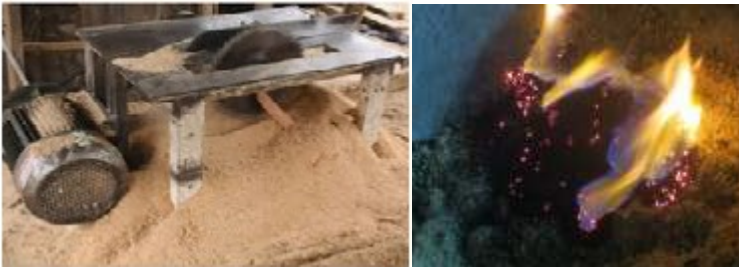
Figure 4: Sawdust burned to become sawdust ash (SDA).
