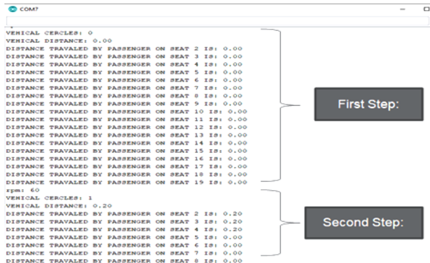
Figure 4.17: Serial Monitor reading for vehicle rpm, Vehicle Circles, vehicle distance and the distance traveled by passengers on each seat
