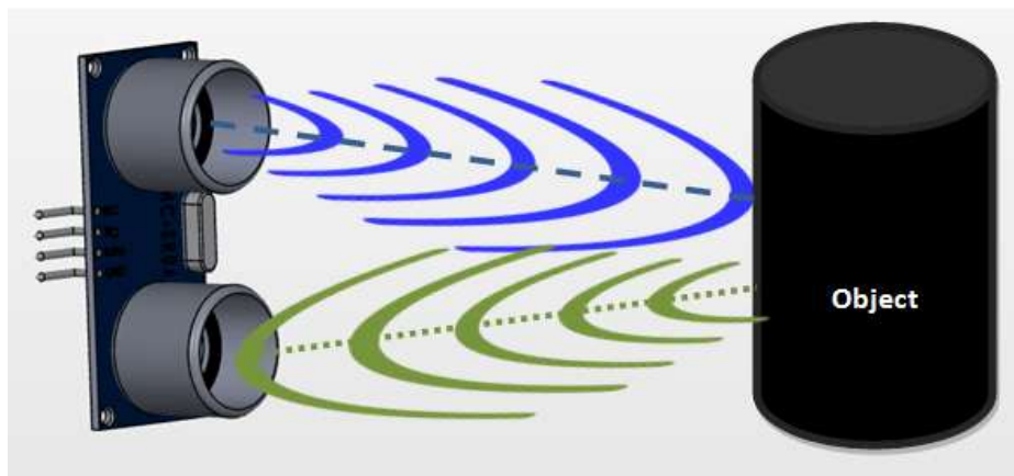
Figure 6: Ultrasonic Sensor principle
