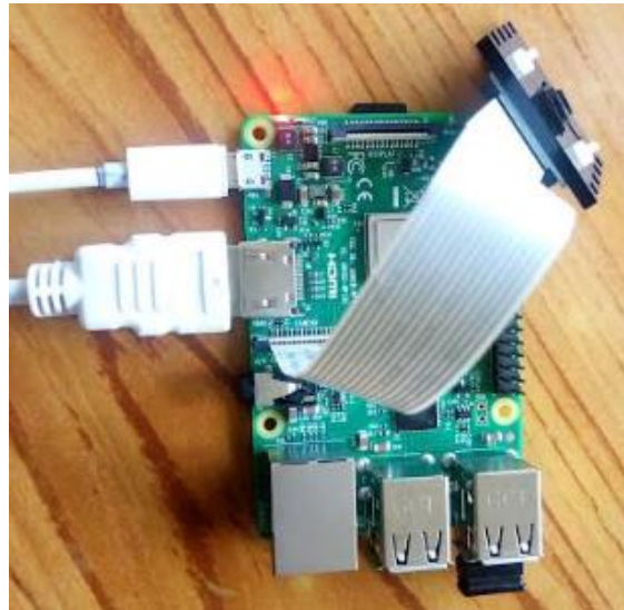
Figure 4. 2: RPi camera connected to raspberry pi
