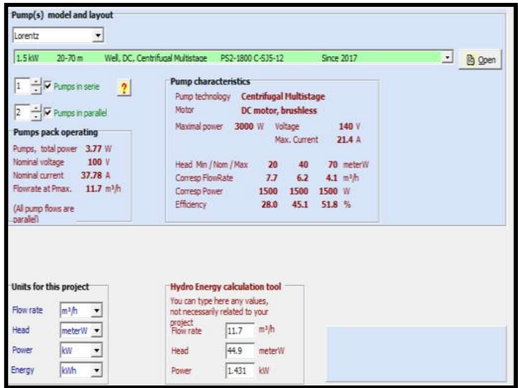
Figure 5-4: system Pump model and layout
