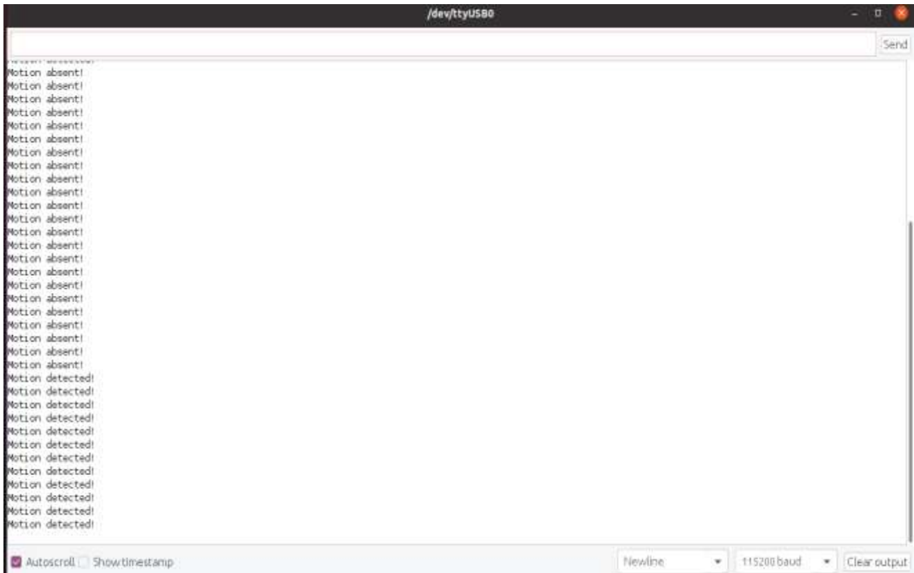
Figure 23: PIR Serial output
