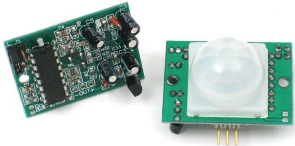
Figure 7: PIR (passive infrared) sensor [26].
