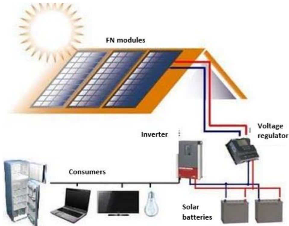
Figure 2.11 Standalone photovoltaic system [3]
