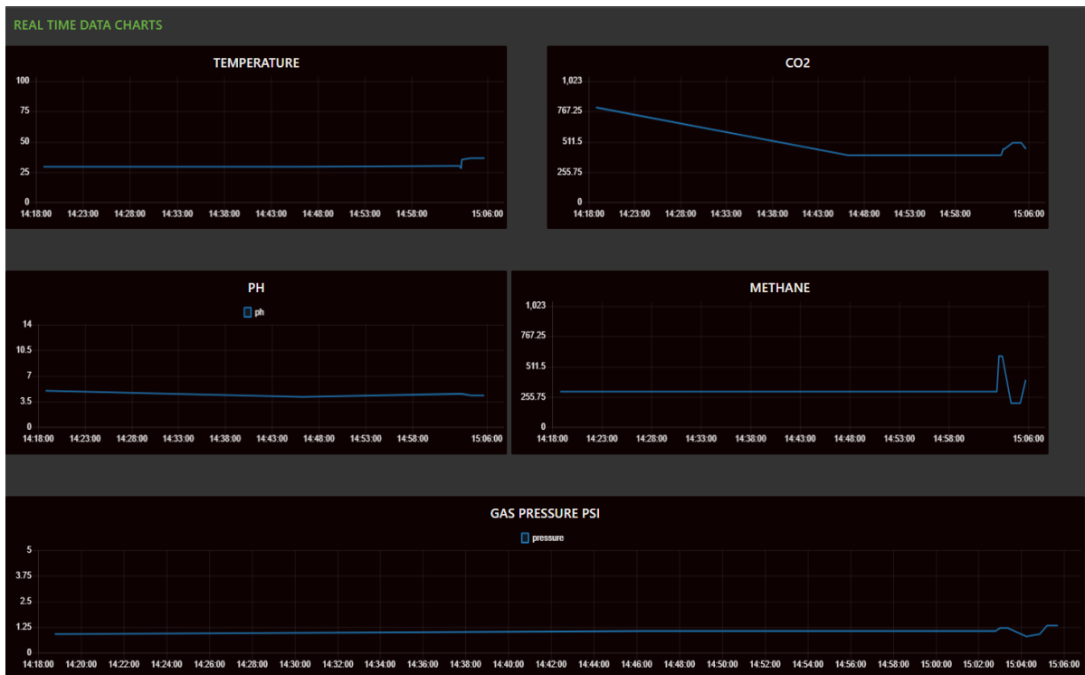
Figure 5.2 Real time data charts on node-red server
