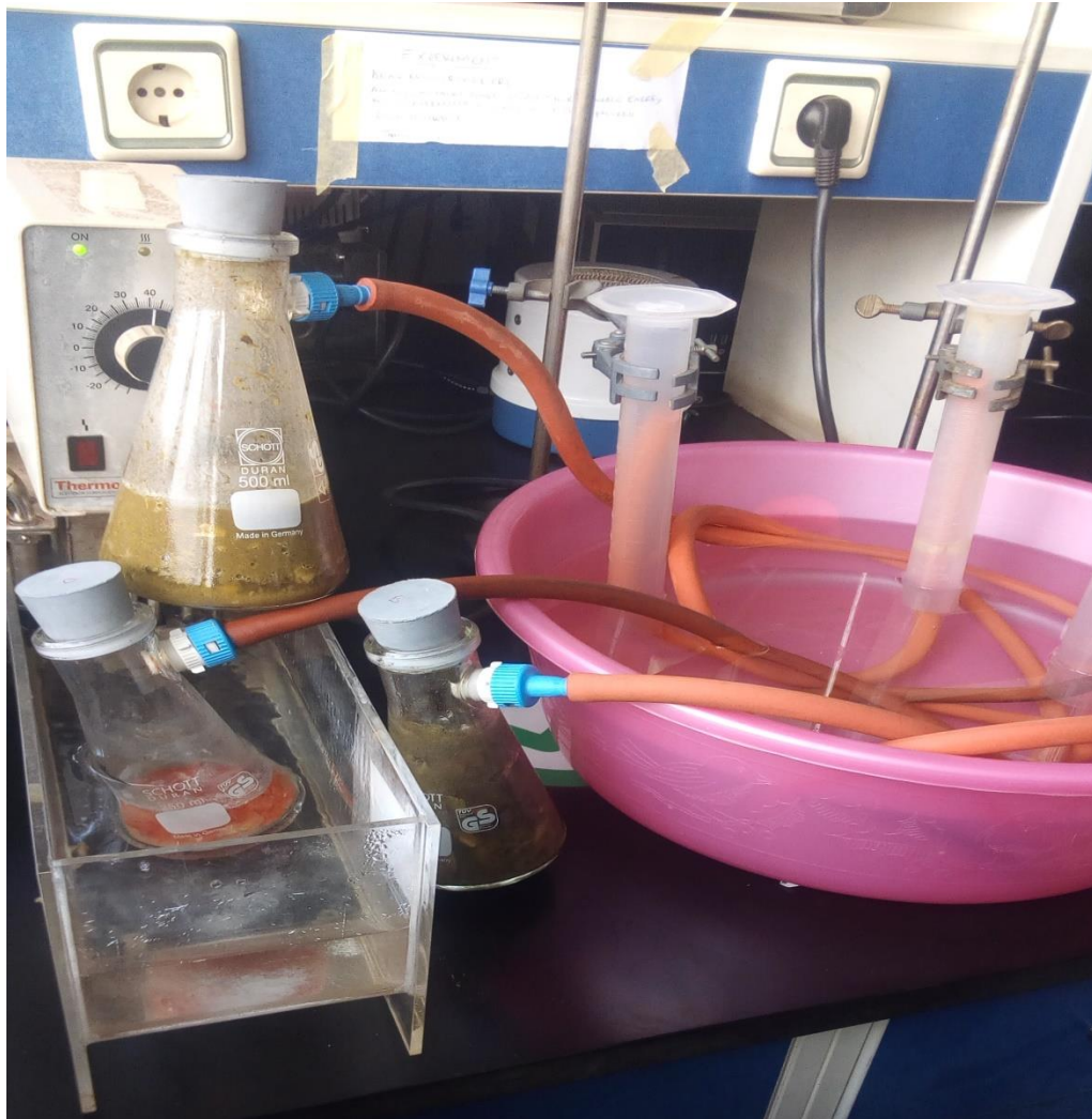
Figure 19: Shows the sample of Biodegradable waste in Erlenmeyer Flask used as Digester.
