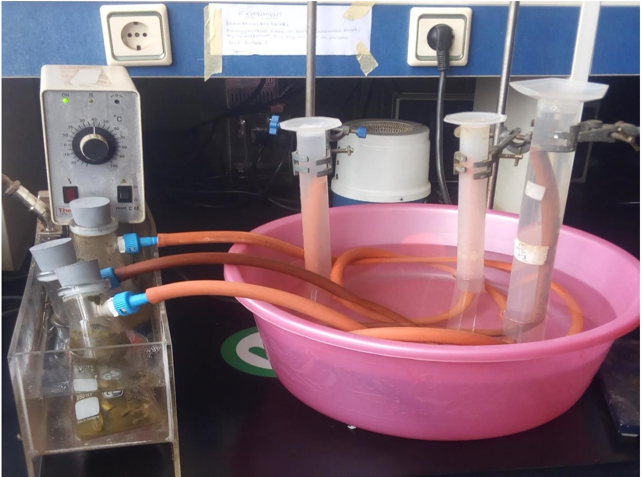
Figure 18: Shows Experiment set-up for biogas production from Biodegradable waste.
