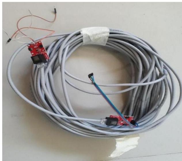
Figure 3.5 The I2C differential interfacing connectors attached to each end of the Cat 6 UTP sensor connection cable (25 m).
