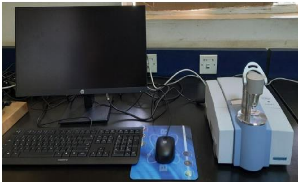
Figure 3: Fourier Transform Infrared Spectrophotometer (Bruker Alpha II, 111311, Germany)
