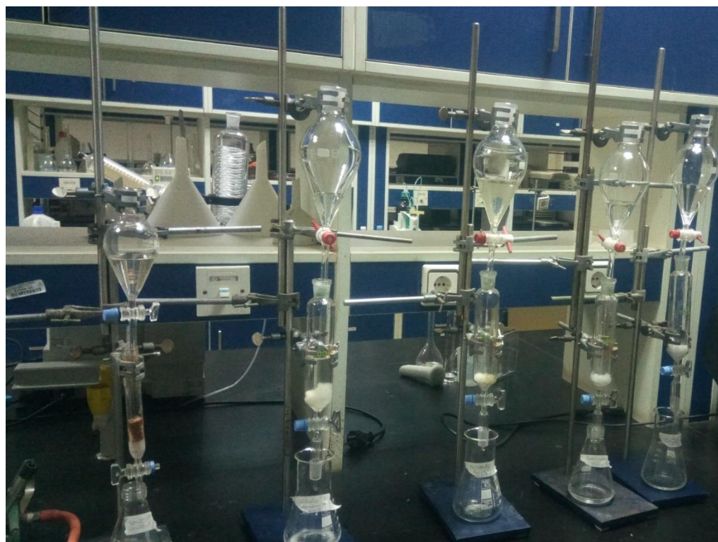
Figure 5: Packed column flow adsorption experiments
