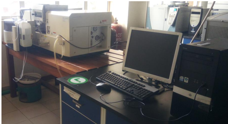
Figure 2: Atomic Absorption Spectrophotometer (AA Shimadzu -6800 with wizard software)
