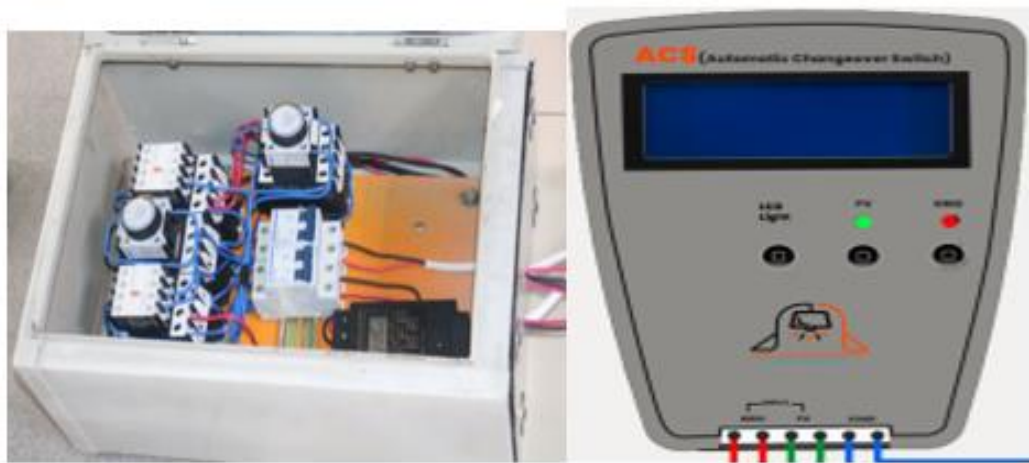
Automatic changeover switch (1) electromechanical, (2) digital
