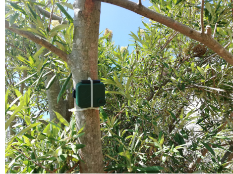
(b) AudioMoth hung at a height of 1.5 meters at a sampling rate of 48 kHz for audio recording.
