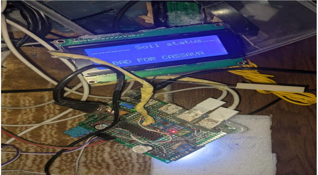
Figure 12: Prototype showing the Quality of the soil
