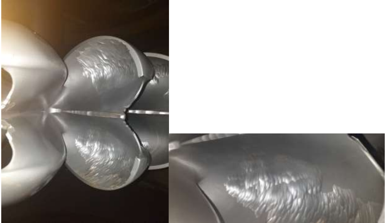
Picture 4.1 Combined effect of sediment erosion and cavitation to the runner blades
