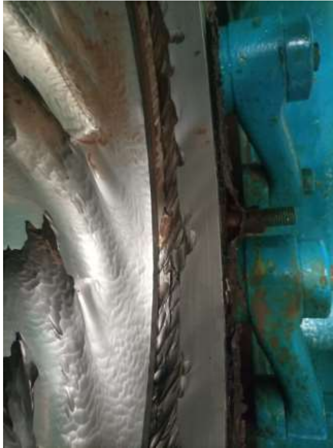
Picture 4.5 Combined effect of sand erosion and cavitation to sealing ring
