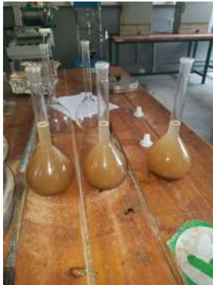
Picture 3.5 specific gravity test
