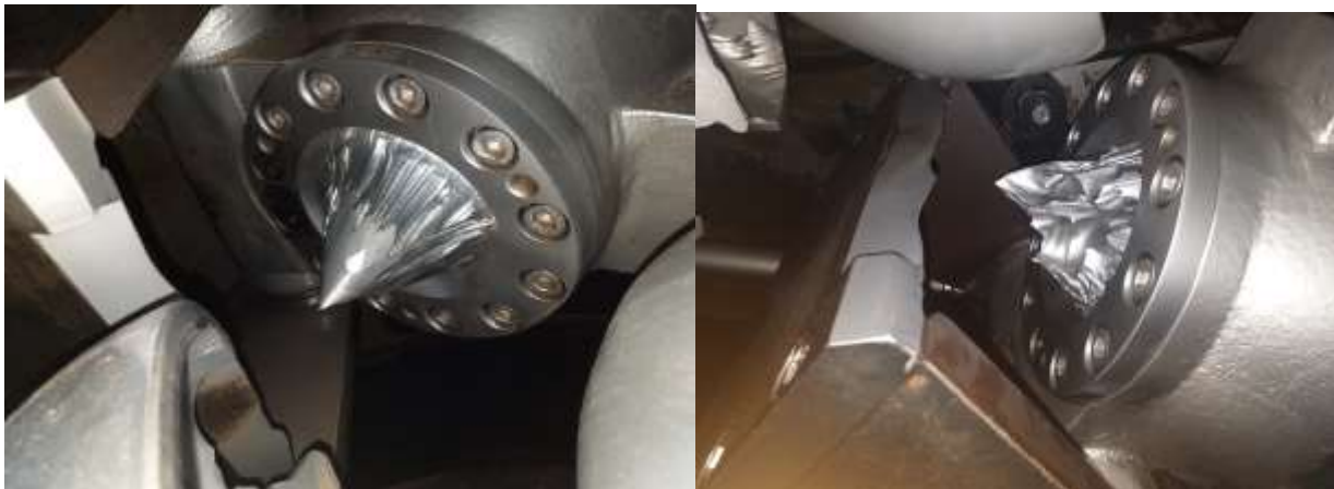
Picture 4.2 Combined effect of sediment erosion and cavitation to the turbine nozzles
