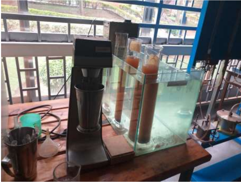
Picture 3.6 hydrometer test
