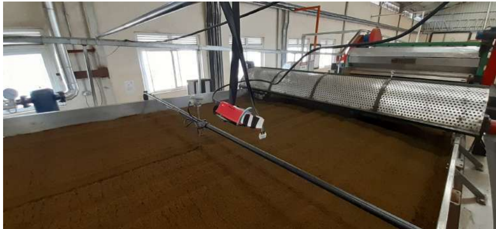
Figure 9.3: Application of Raspberry Pi 3 Model B+ with the Pi camera for taking pictures during the fermentation of black tea in the Sisibo Tea Factory, Kenya.
