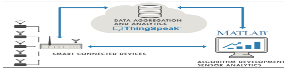
Figure 4. 17: ThingSpeak cloud block diagram
