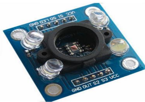
Figure 4. 8: TCS3200 Color Sensor
