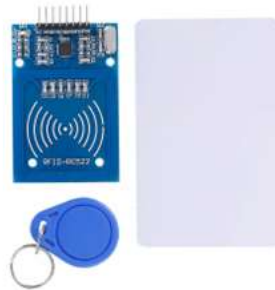
Figure 10: RFID Reader module
