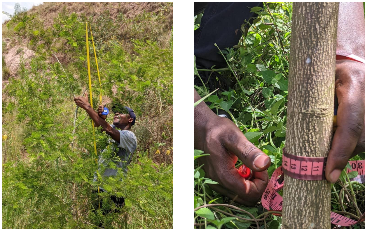
Figure 5. Field measurement of height and base-diameter of trees
