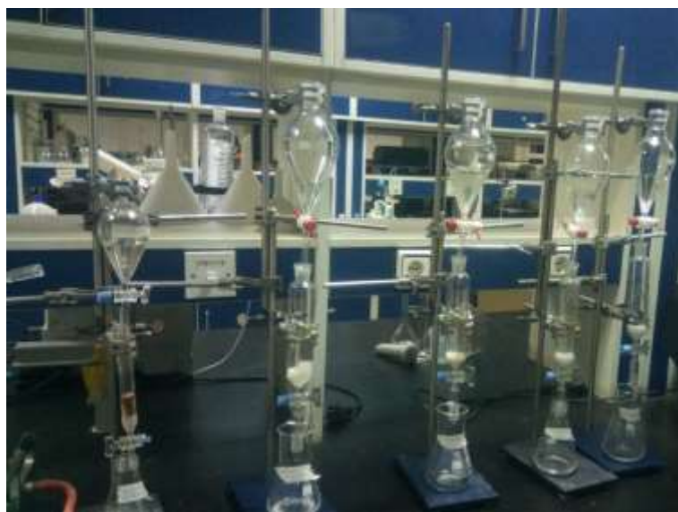
Figure 3: Experiments on adsorption in packed beds
