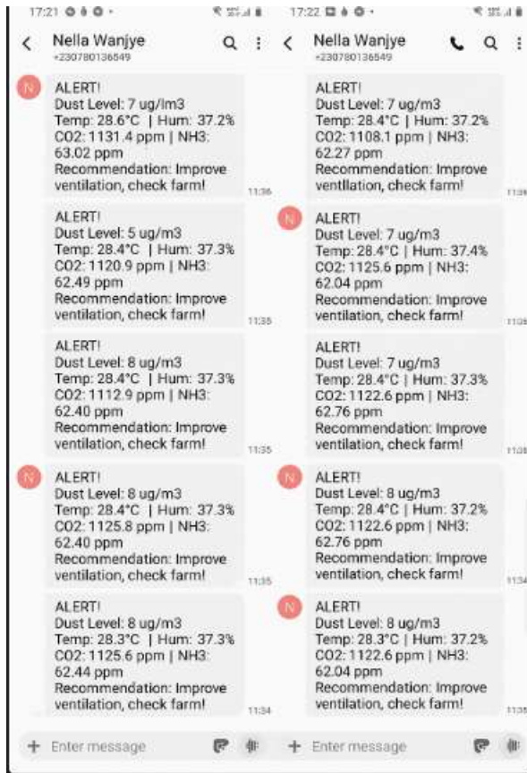
Figure 11: Screenshot of SMS alert message received on farmer’s phone during real-time environmental threshold violation.
