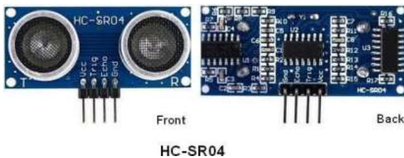
Figure 9: HC-SR04 Pin Diagram
