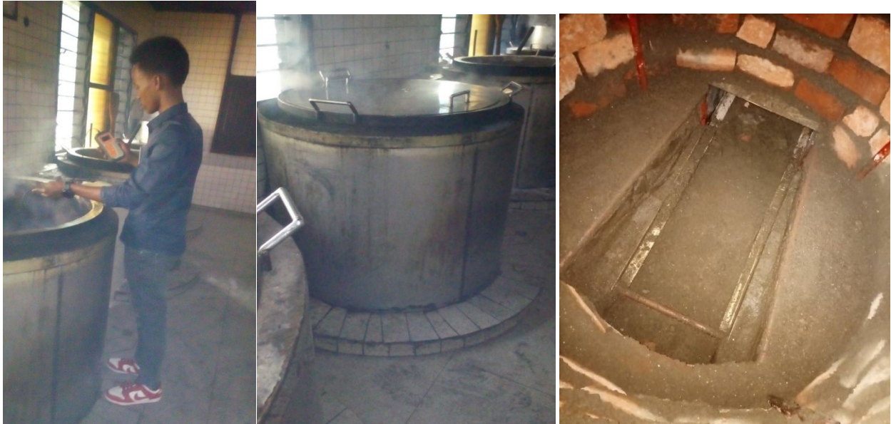
Fig A.1 Data recording on field (a), final manufactured stove model (b), and construction chamber model (c) of Community Stove at RP IPRC Tumba Colledge.
