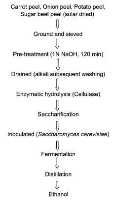
Fig. 1 — Flow diagram for production of ethanol using cellulase enzyme
