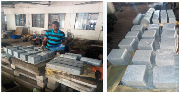
Figure3.10 Curing of concrete specimens by external self curing method
