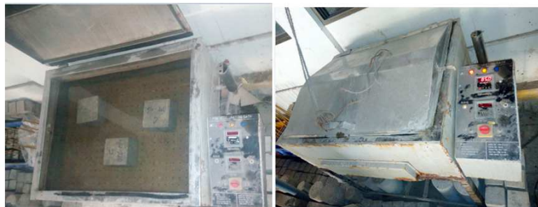
Figure 3.16 Saturated mass by using immersion in boiling water at 85 o c
