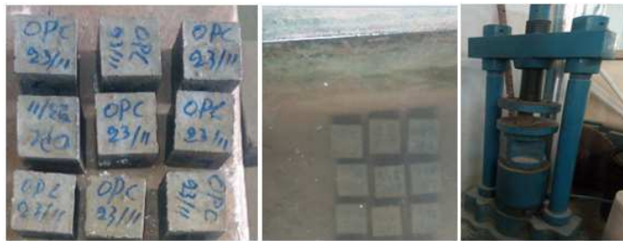
Figure 3.1 Preparation and testing of compressive strength of cement paste for OPC
