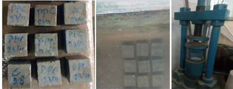
Figure3.2 Preparation and testing of compressive strength of cement paste for PPC
