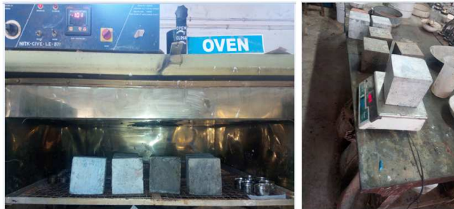
Figure 3.14 Oven-dry mass of samples for concrete water absorption
