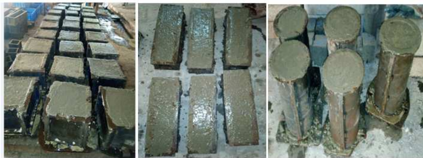
Figure3.7 Casting of the concrete specimens
