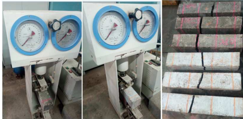
Figure3.13 Testing of concrete flexural strength
