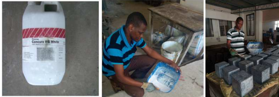
Figure3.3 Preparation and application of Concure WB curing compound
