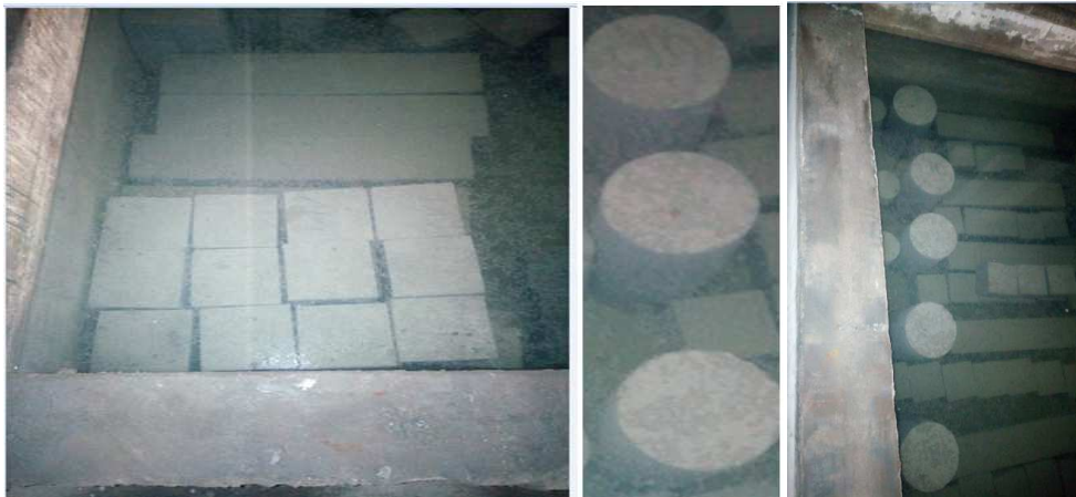
Figure3.9 Curing of concrete specimens by conventional curing method
