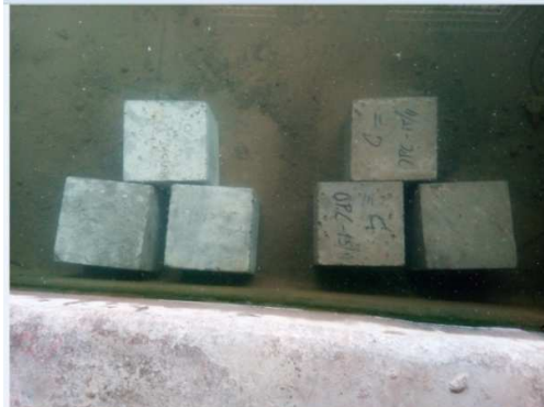
Figure 3.15 Saturated mass of samples for concrete water absorption
