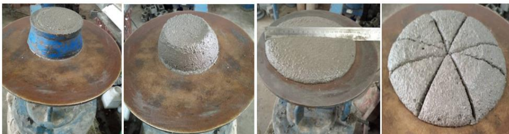
Figure 4. 9 Fresh steel fiber geopolymer mortar subjected to mini flow table test
