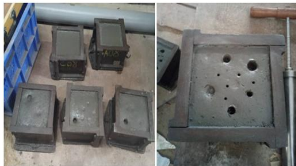
Figure 4. 1 Sample tested using penetrometer
