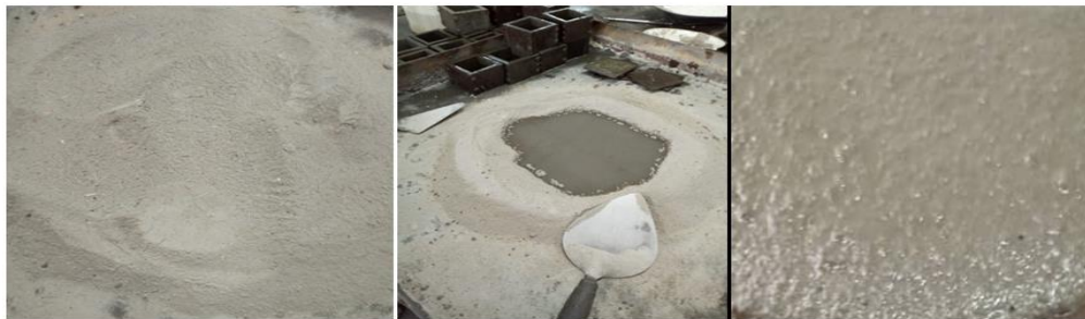
Figure 3. 10: Steel fiber geopolymer mortar preparation and some specimens
