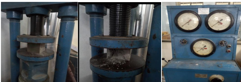
Figure 3. 12 Sample subject to compressive machine
