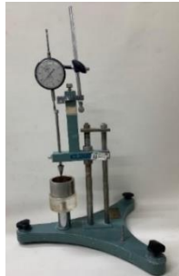
(b) Liquid limit cone penetrometer apparatus
