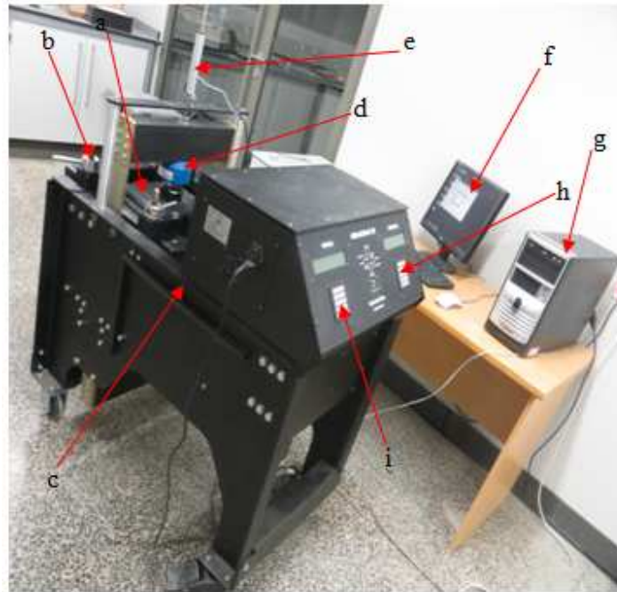
Figure 3.3: Automated large ShearTrac-III system (Various components of ShearTrac-III (a) Shear box, (b) Screws, (c) ShearTrac-III frame, (d) Vertical load cell, (f) Computer screen, (e) Vertical displacement transducer, (g) Computer monitor, (h) horizontal front panel controller and (i) Vertical front panel controllers (Geocomp Corporation, 2012)
