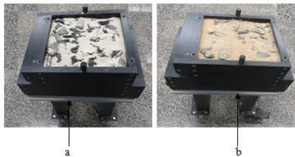
Figure 3.8: Prepared test specimen in shear box for (a) Cape Flats and (b) Klipheuwel sand-shreds mixtures for 50-60 mm tyre shreds
