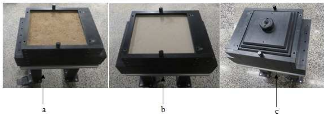
Figure 3.6: Prepared test specimen in shear box for pure sand (a) Klipheuwel sand, (b) Cape Flats sand and (c) the sealed sample in the shear box with top cap
