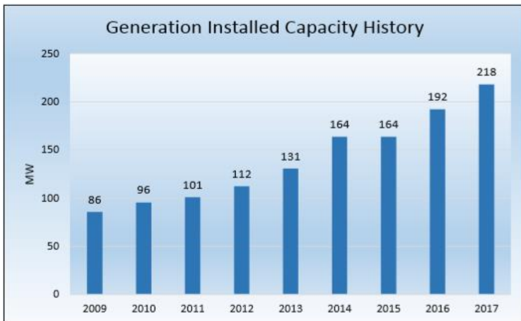
Figure 1: The evolution of installed electricity generation capacity of Rwanda
