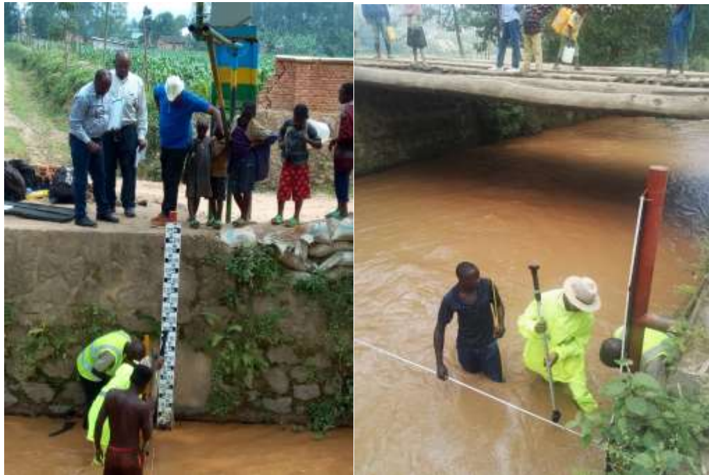
Fig. 3.3 Taking point velocities for discharge measurement using a currentmeter
