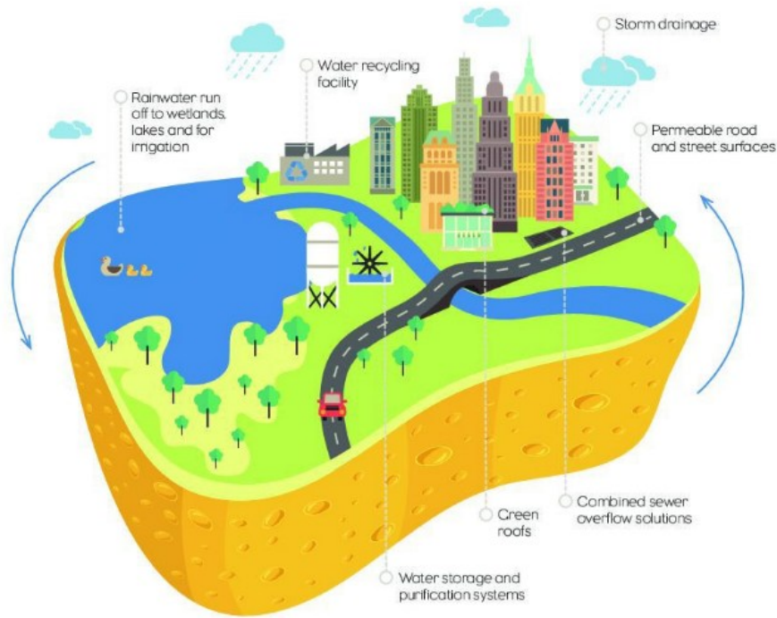
Figure 4 Schematic diagram of the Sponge city concept
