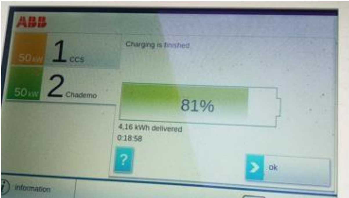
Figure 21: Charging process from the grid
