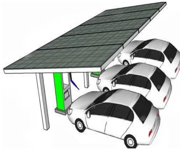
Figure 13: The example of solar powered charging station for electric vehicle
