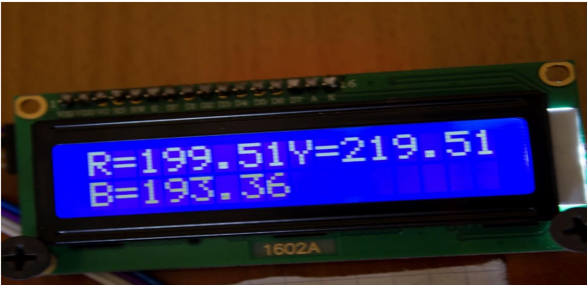
Figure 4. 16:: Shows Voltage Imbalance due to Unbalanced Load
