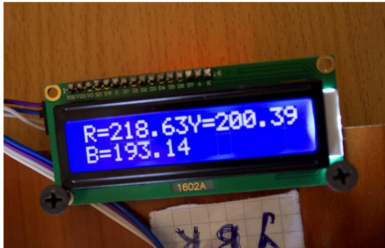
Figure 4. 13: Message shows that Red Phase is missing
