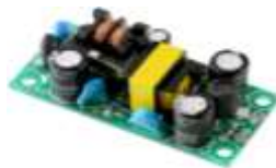
Figure 3.10: AC-DC Power Supply
