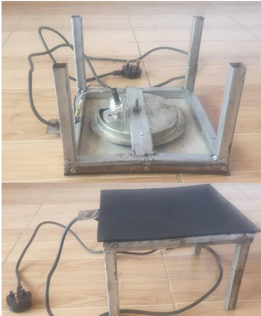
Fig. 4. 6: Warmpak heating table with all its components
