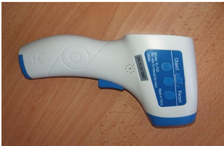
Fig.4.8: Special surface thermometer to measure the temperature for both the warm pak.
