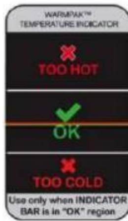
Fig.4.4:Temperature display unit at the operating state of ok.
