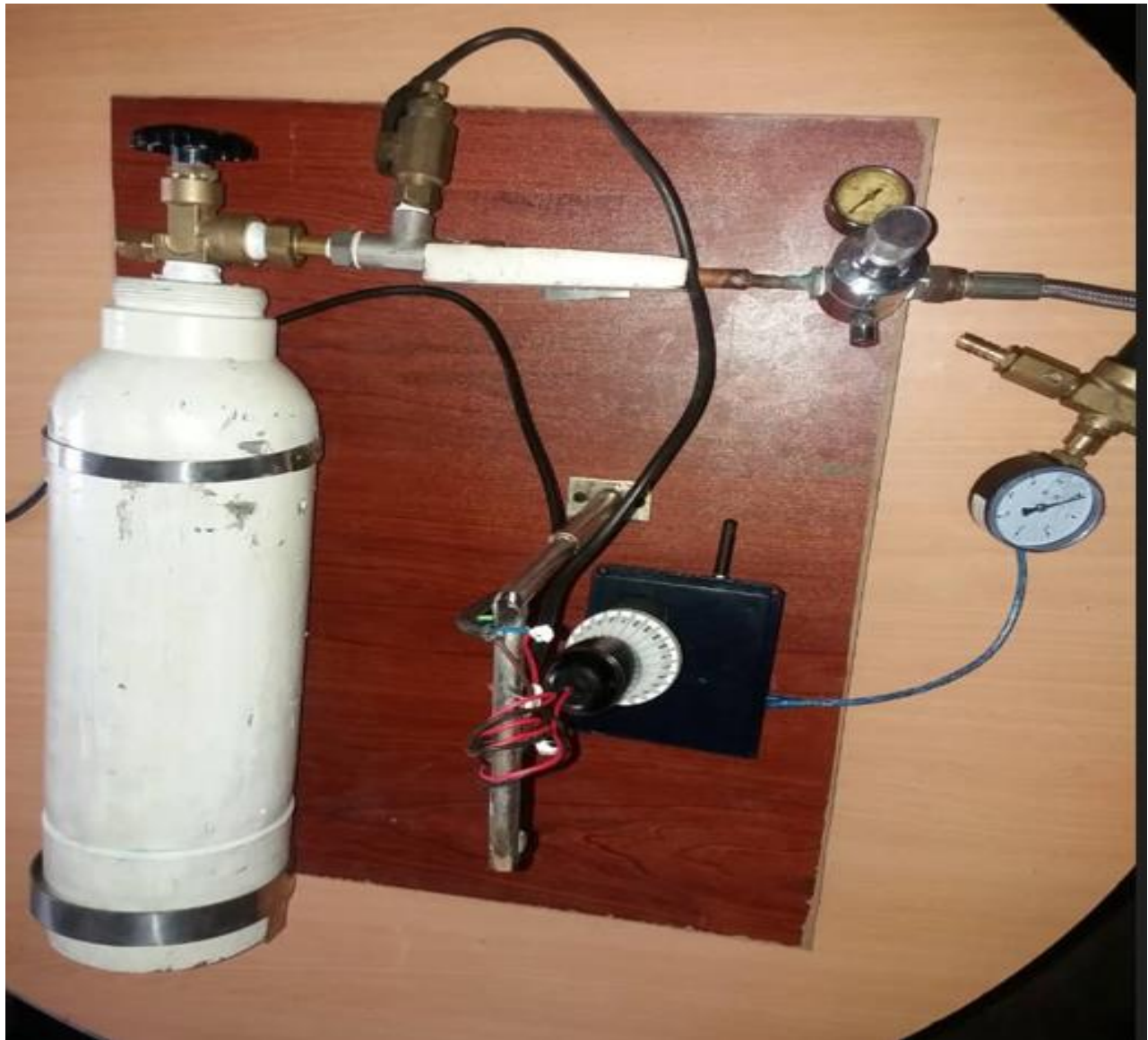
Figure 4.18 Entire functional circuit of IoT based medical oxygen monitoring system in ICU
