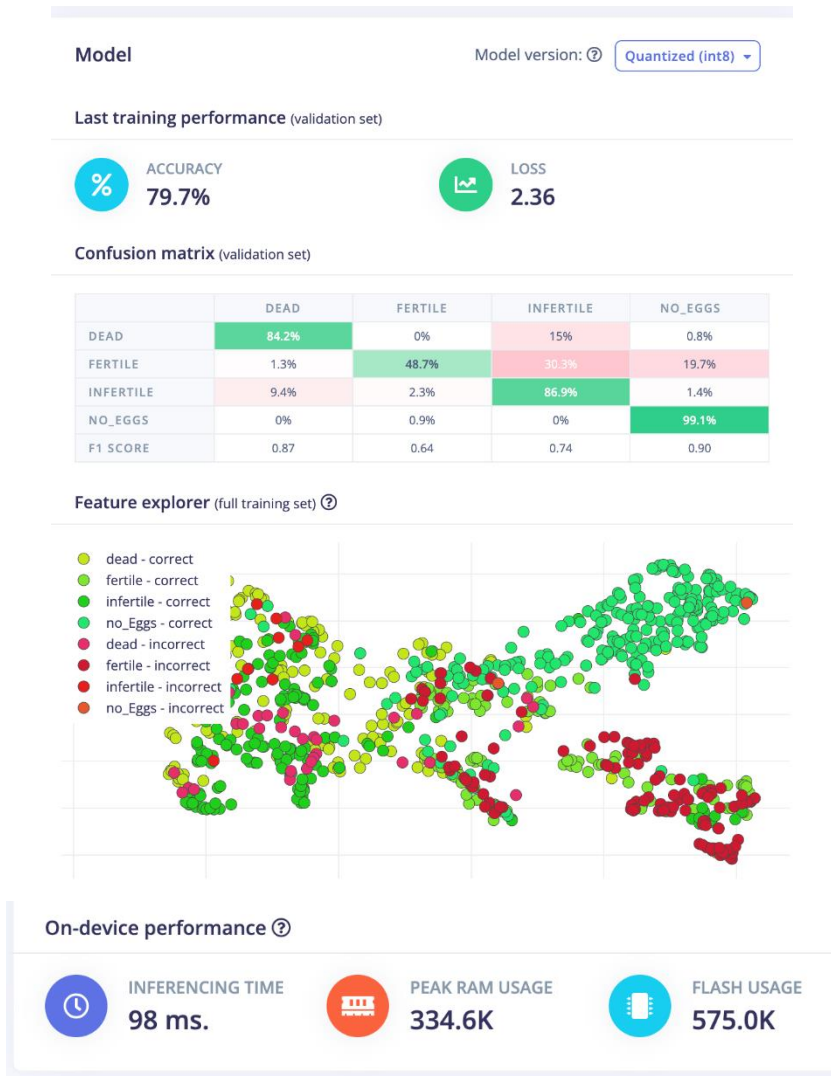
Figure 36: Model training results in quantized version using MobileNetV2.
