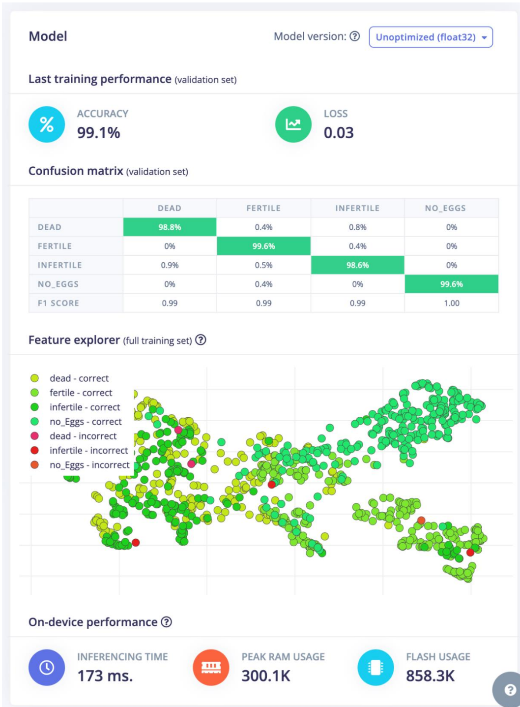
Figure 38: Model training results in unoptimized version using MobileNetV1.
