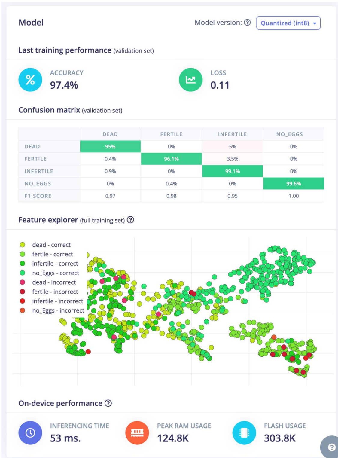
Figure 39: Training result in quantized(int8) version using MobileNetV1.
