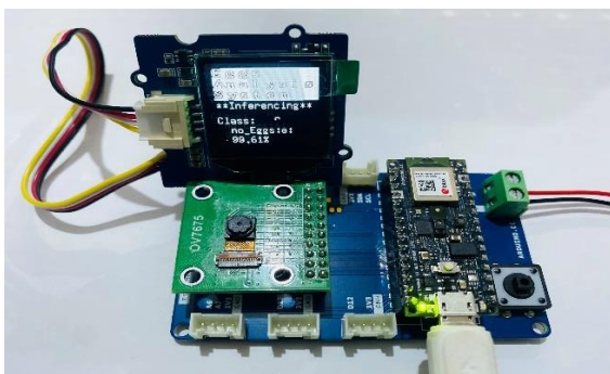
Figure 28: OLED and camera connected to Arduino nano 33 ble sense
