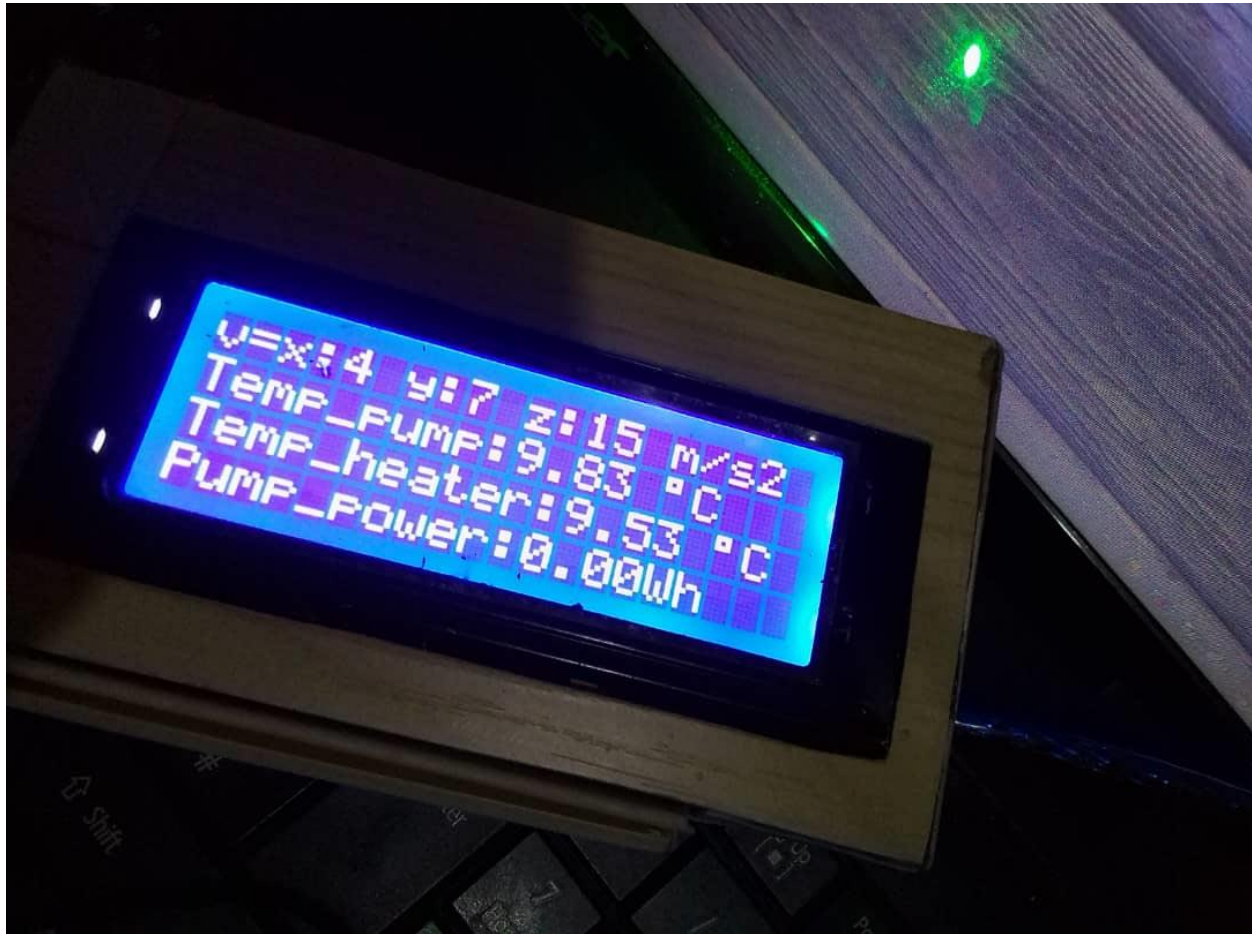
Figure 4. 4: System displaying sensor readings
