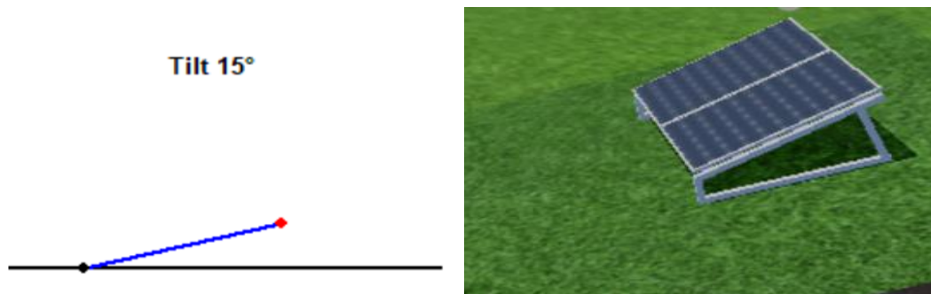
Figure 4. 1 Tilt angle at which solar panels are mounted to face the sun on the selected site
