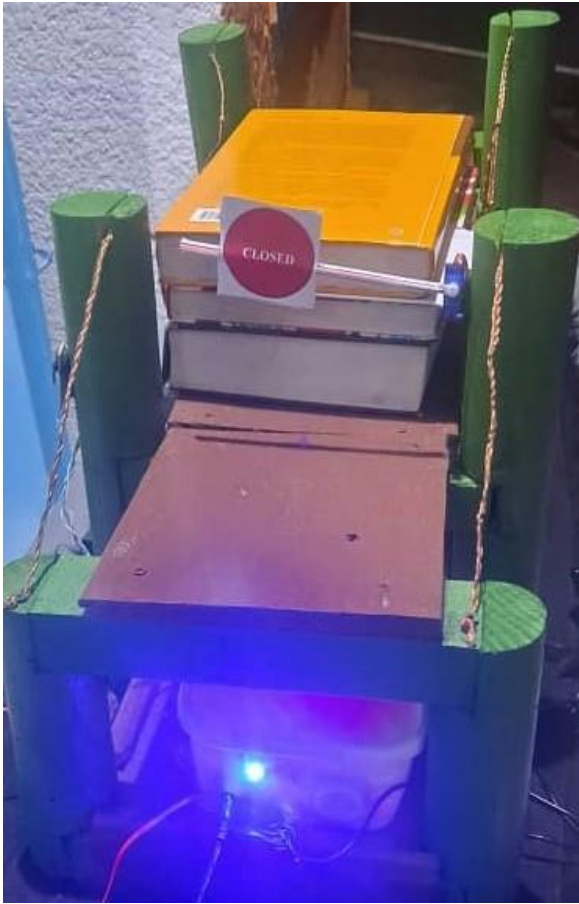
Figure 28:Overweight scenario (Blue LED ON and Bridge closed)
