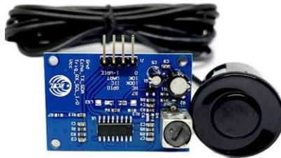
Figure 12:Water proof Ultrasonic Sensor
