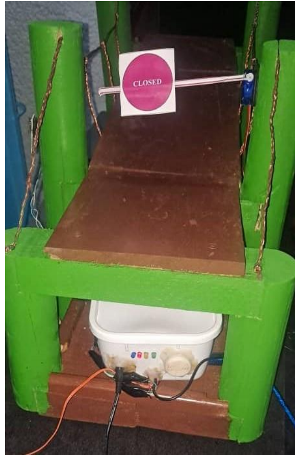
Figure 27:Flooding senario (Red LED ON and bridge closed)
