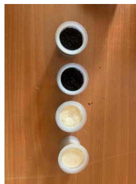
Figure 4.17: 4 tubes with 2 samples (Sago seed powder raw material (Black) and Sago seed Activated carbon (white))
