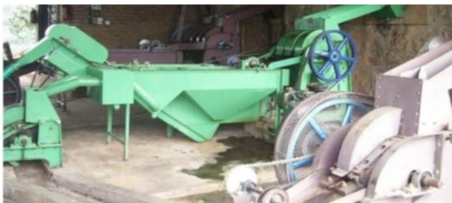
Figure 1.4: Machine used to remove the core of Coffee
