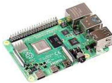
Figure 3.7 Raspberry pi 4 8GB Ram
