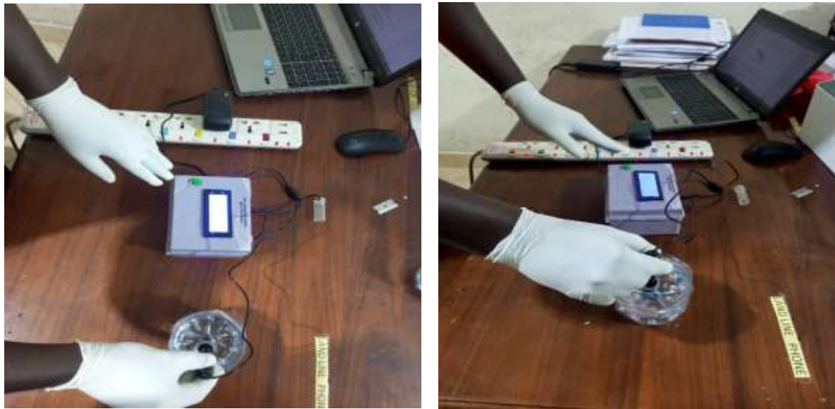
Figure 18: Inserting Acetylcholinesterase bio-sensor into water compound and into organophosphate compound.
