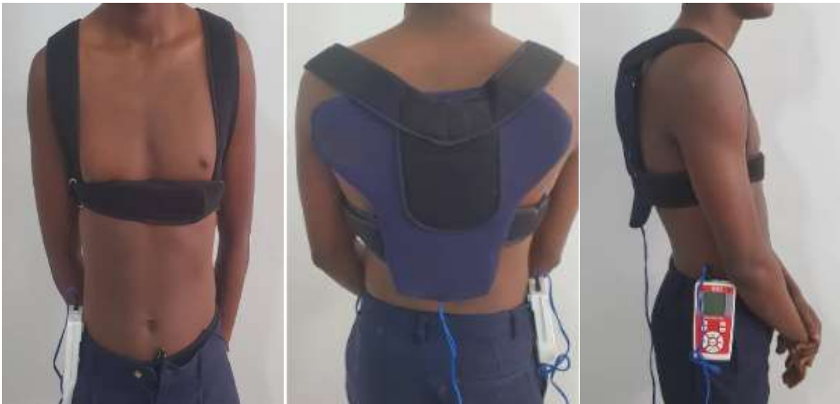
Figure 4.3. Wearable spine posture and shoulders corrector with TENS Machine
